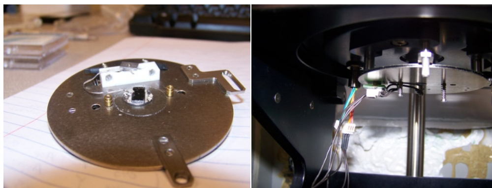
Figure 4. A typical installation of the sample for EFM and KFM measurements. Left – a piece of graphite with organic layer as a sample with grounding wire attached to the sample with a drop of conducting silver glue. Right – a grounding connection under the sample plate.
