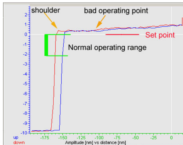
Fig. 6.6 Amp-distance curve showing 'Normal operating range'
